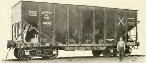
An American Steel Hopper-bottom Coal Car
